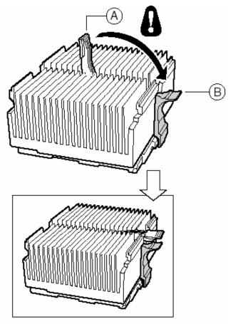
Figure 19: Locking Heatsink Lever
